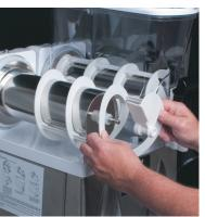
4.Pull the auger from the cooling drum.
