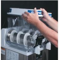
1. Unplug the hopper lamp cord(s) 2. Depress the hopper lock plunger, 3. Pull the hopper assembly forward and remove the hopper lid(s). lift slightly. **NOTE:** On Autofill models, remove the level probe and fill tubes from the hopper.
