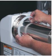
5. Remove the hopper seal from the flange on the cooling drum.
