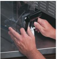
6. **CAUTION:** Faucet valve is under 7. Carefully slide valve up to remove 8. Remove the auger nose bushing 9. Remove the drip tray and cover. spring tension. Spread one side of spring and faucet seal. Extra care from inside the front of the hopper. the handle first, then the other and should be taken when handling the NOTE: Do not scratch this surface disconnect from hopper.
