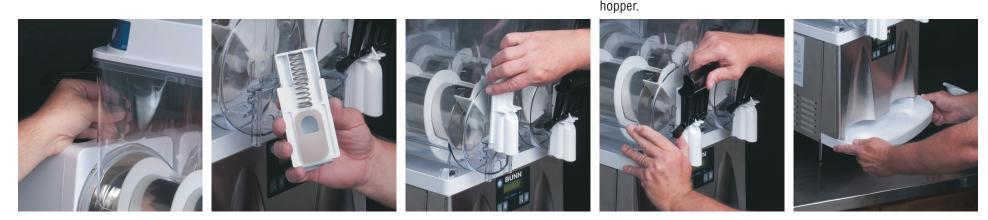
7. Plug in the hopper lid lamp 8. Position the faucet seal and the 9. Slide the faucet valve assembly cord.
