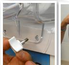
Remove the spiral blade assembly and suction cap gasket by removing the retaining knob.
